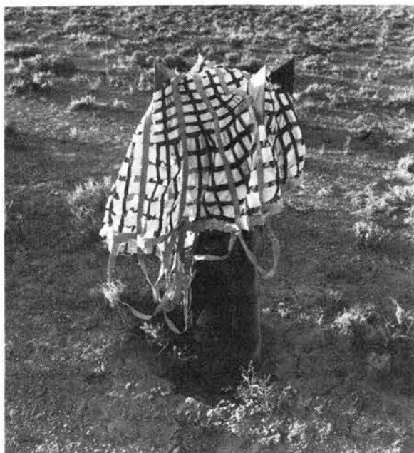
TOP PHOTO shows Honest John rocket ready to launch test payload from Tonopah Test Range. Payload carries a 5-foot (diameter) parachute that can survive deployment at Mach 2 (twice the speed of sound); see photo on Page One. Bottom photo shows payload after impact; obviously, the chute survived.
